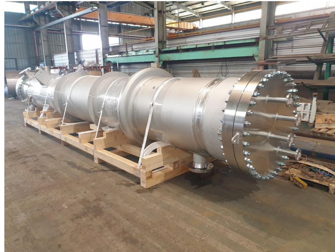
White Liquor Heater Designed for heat exchange of highly viscous white and black liquors.(2020)
