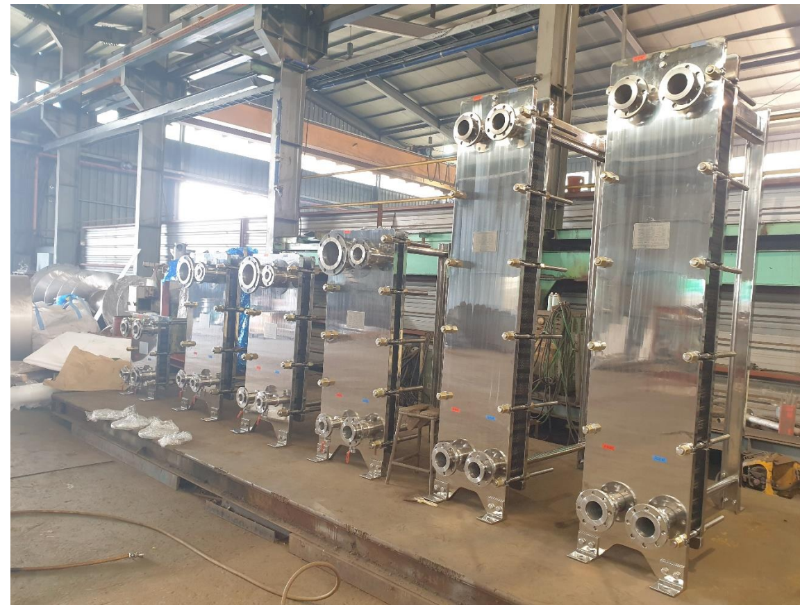
Plate Heat Exchanger Plate Material: C-276 HASTELLOY Gasket Material: Viton (2020)
