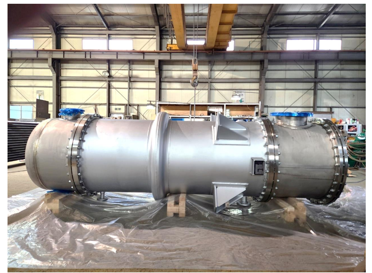
Titanium Heat Exchanger Designed and manufactured MC and DMAC heat exchangers with Ti Gr.2 material. (2024)
